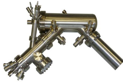
FIG. 5: Photograph of the FERRUM spin detector mounted (at the left hand site) at the exit flange of a cylinder sector analyzer CSA 300. The analyzer entrance lens (right) is covered by a protection cylinder. The analyzer mu-metal chamber is directly connected to the detector double mu-metal shielded chamber. The Fe-deposition source and the thermal oxygen doser are integrated with the detector housing. Because of the 90 deflection of this analyzer no additional deflector is needed to measure in- and out-of-plane spin components.
