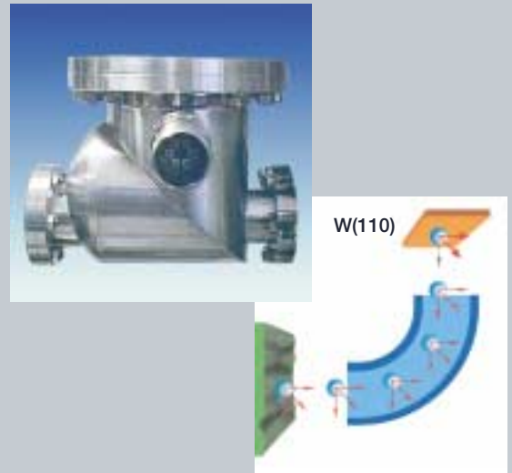
Using a 90° deflector, spin vector components parallel and perpendicular to the surface can be detected simultaneously after 90° deflection of the emitted electrons as illustrated.
